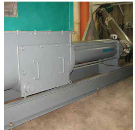
Easy maintenance through large inspection cover.
