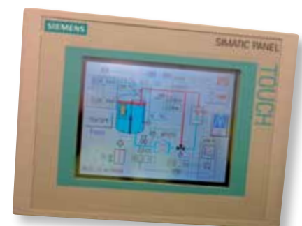
▲ An operator panel is used to run the plant locally. It is connected via, for example Profibus, to the master control system.
